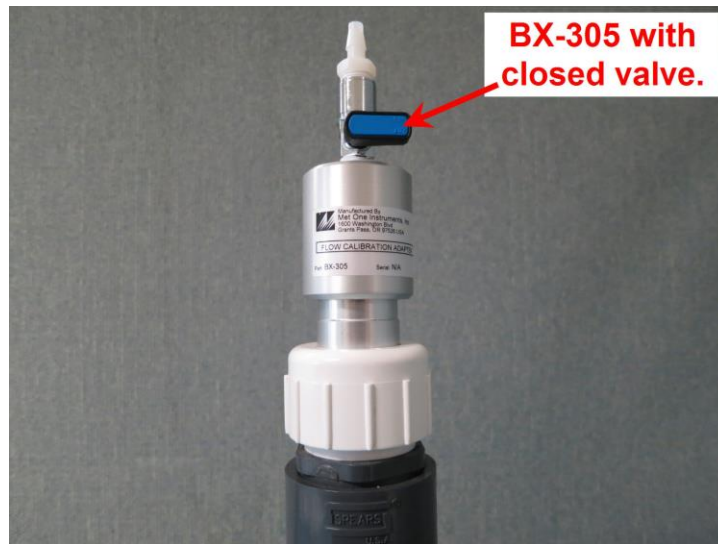
Figure 6-2 BX-305 Installed on Inlet Tube
