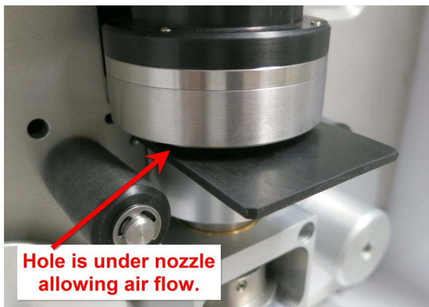
Figure 6-6 Nozzle Sealing Tool Upper System Test Configuration
