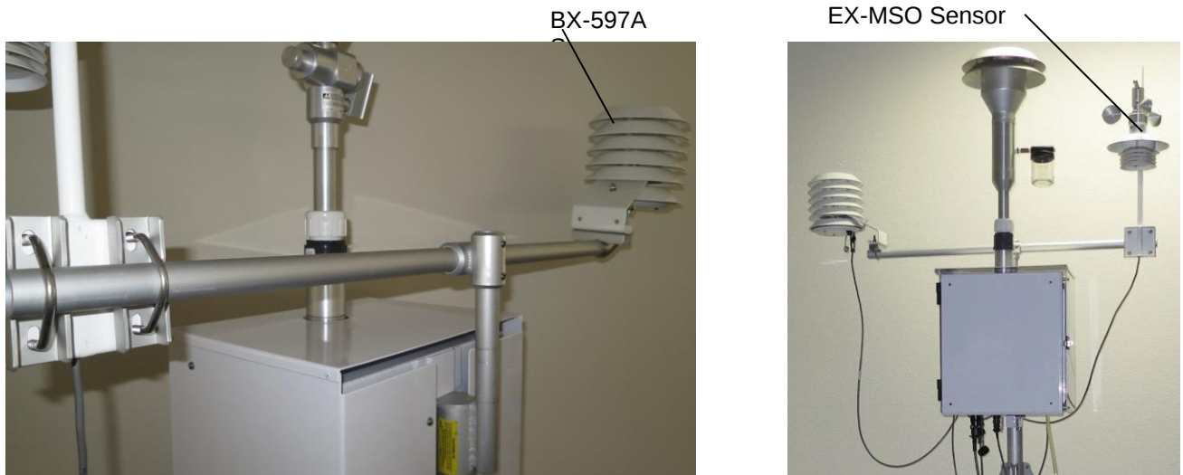
Figure 2-4 Sensor Mounting with an Optional Wind Sensor
