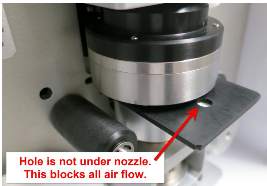
Figure 6-5 Nozzle Sealing Tool Lower System Test Configuration
