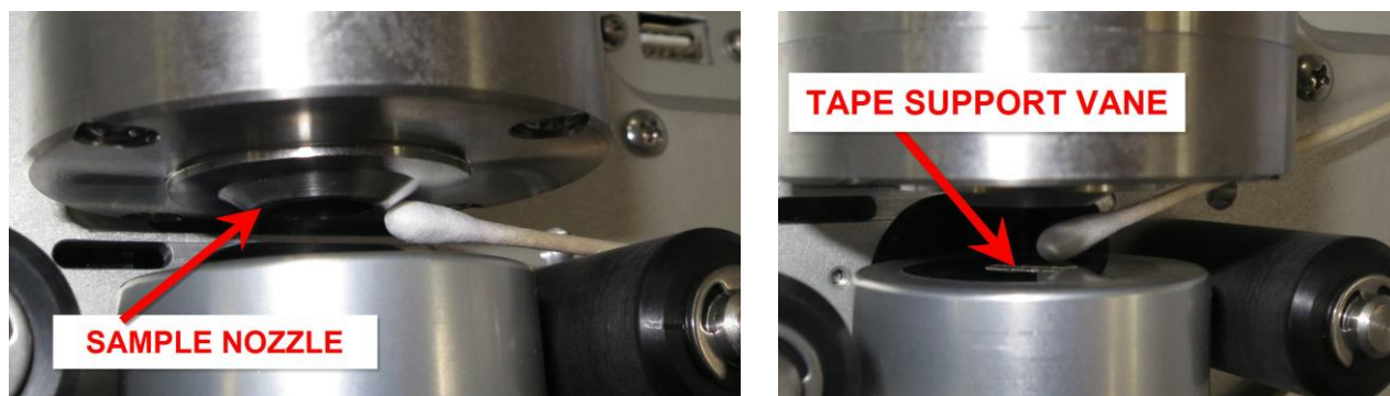
Figure 6-8 Cleaning the E-BAM PLUS Nozzle and Vane with a Cotton-Tipped Applicator
