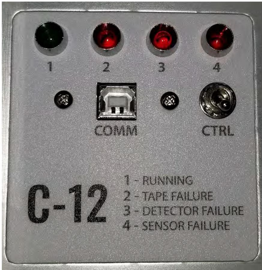
Figure 6-1 LED and Toggle Switch Interface
