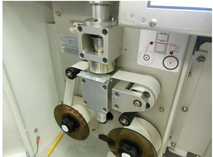
When the zero foil is detected, the nozzle will automatically lower on to the foil and the four minute measurement will commence. After four minutes, the nozzle will be raised, and the screen will instruct you to remove the zero foil. Remove the zero foil. Take care to minimize tape movement.
