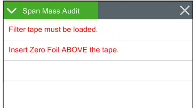
Insert the zero foil **above the filter tape** between the nozzle and vane, with the label facing up. Take care to minimize tape movement.
