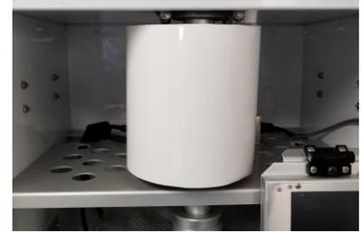
8. Slide the inlet tube through the pipe seal on top of the enclosure just until you can see it inside the enclosure. Position the inlet heater beneath the inlet tube and slide the tube through the heating element until it just comes in contact with the O-rings. Raise the heater so it is near (but not touching) the top of the enclosure and fasten it in position with the supplied hex wrench. See image above center.
