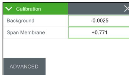
The Span Membrane is the factory-set expected mass of the reference membrane foil. Each unit's span membrane value is different, but is typically near 0.800 mg/cm<sup>2</sup>. Refer to the BAM 1022 calibration certificate that comes with the BAM 1022. The span membrane value will be listed under the Span Audit Value. **The span membrane value is never changed by the operator unless the span membrane foil is replaced due to damage.**
