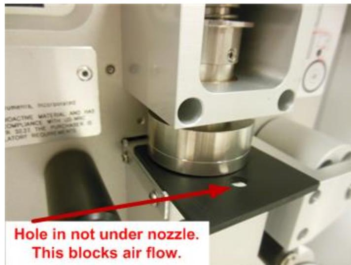
3. Press the LEAK ON button. The BAM 1022 will start the pump and begin the leak test.
