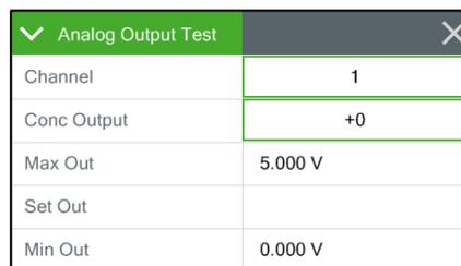
You'll notice the Min Out and Max Out fields match the zero and full scale values for the selected output. Between them is the Set Out field, which will update with the expected output based on the concentration selected. Verify the output on the back of the BAM 1022 matches the Set Out value shown.
