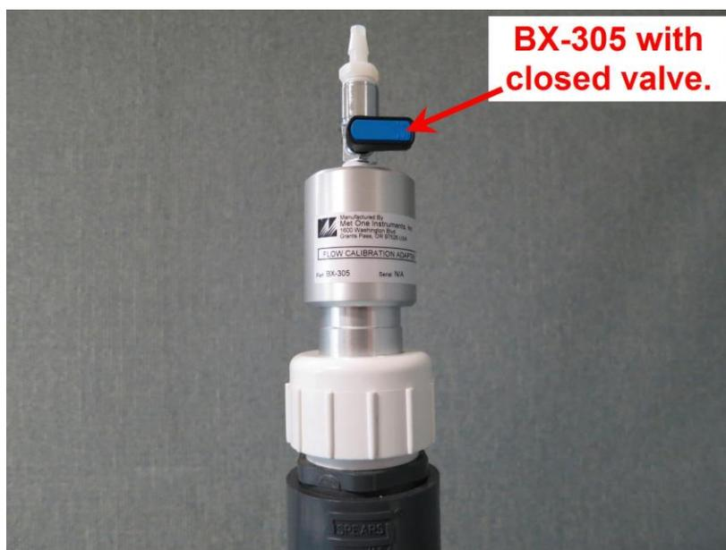
10. The pump flow rate should drop below 1.5 LPM.
