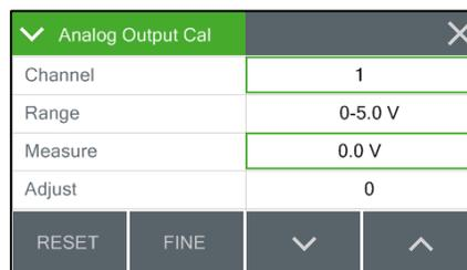
After selecting the output channel, the measure field may be adjusted to maximum or minimum value and the output of the channel confirmed. Just tap the green bordered Measure box and select the desired test output. Verify the actual output using a voltmeter at the appropriate channel terminals on the rear panel of the BAM 1022.
