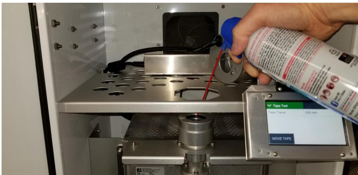
5. Go to the Operate menu and select Start Sample to start a new sample. Allow the pump to run for approximately 1 minute and then stop the sample.
