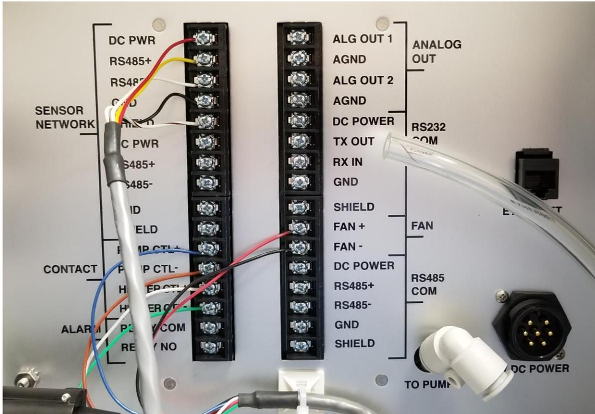
The BX-597A Digital Sensor connects to the top sensor RS485 Sensor Network terminal connections. The second set of RS485 terminal connections is for an optional wind sensor, if used (see section 10.2).
