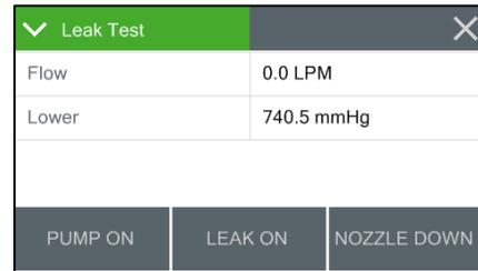
Use the LEAK ON button to lock the flow controller at its current value. This forces the flow controller not to change regardless of blocking the flow or not.
