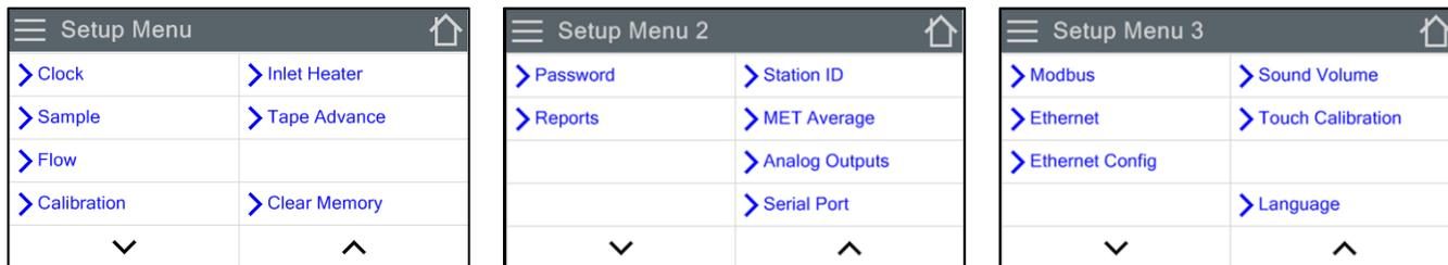
Note that the display has a limited amount of space and cannot show all options on one screen. Tap the up and down arrow keys to navigate between the screens shown above.
