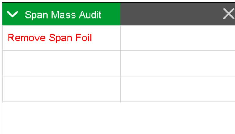
Remove the foil and the display will automatically return to the Test menu.
