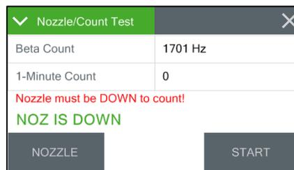
Counting should only occur when the nozzle is in the down position.
