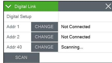
**Scanning for Sensors in the Digital Setup Screen**
