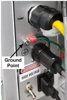
13. Install the AC power supply cable to the remaining connection on the bottom of the internal power strip. It is located next to the ON/OFF switch. See photo above right. Route the power cable and the sensor cable out of the bottom of the cable access opening.
