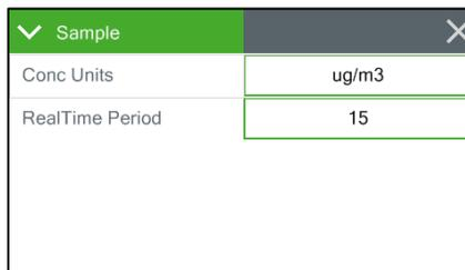
The Data Average (see section 3.5.12) must be set to an interval less than or equal to the Real Time Period in order to properly log the Real Time values.
