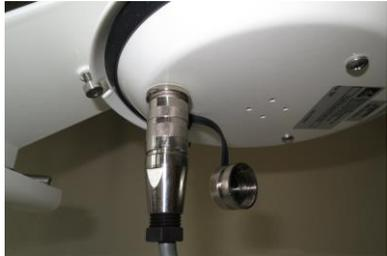
12. Route the sensor cable to the back of the enclosure and attach it to the SENSOR NETWORK terminals in the top position see below left table and center photo.
