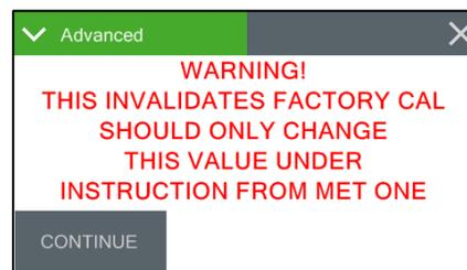
Pressing the 'Continue' button will allow the user into the Advanced screen, where users may adjust the K-Factor Calibration Constant. Only change this setting with advice from the factory.
