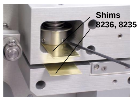
Using Shims for Reassembly
