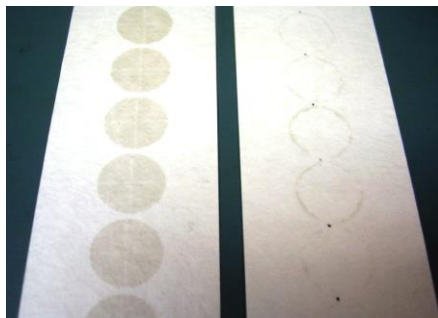
BAM-1020 hourly filter tape spots
