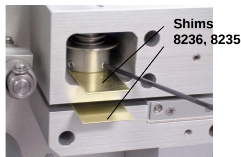
Using Shims for Reassembly
