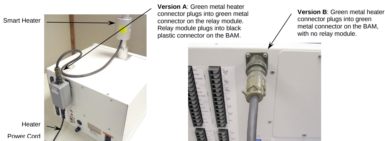
Two Different Smart Heater Power Configurations
