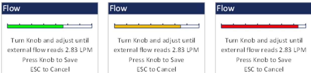
**Figure 17 - Flow Screen Progress Bar Color Changes**
